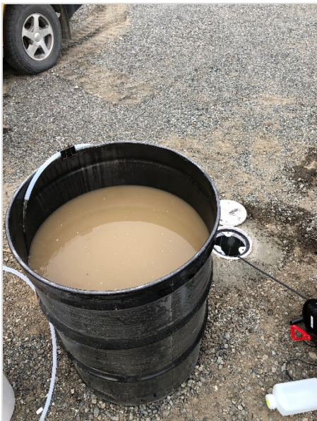
Exhibit 2-4: Groundwater MW purging prior to sample collection.
